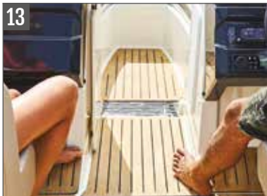
Unique bow drain system avoids water to accumulate and flow into the cockpit
