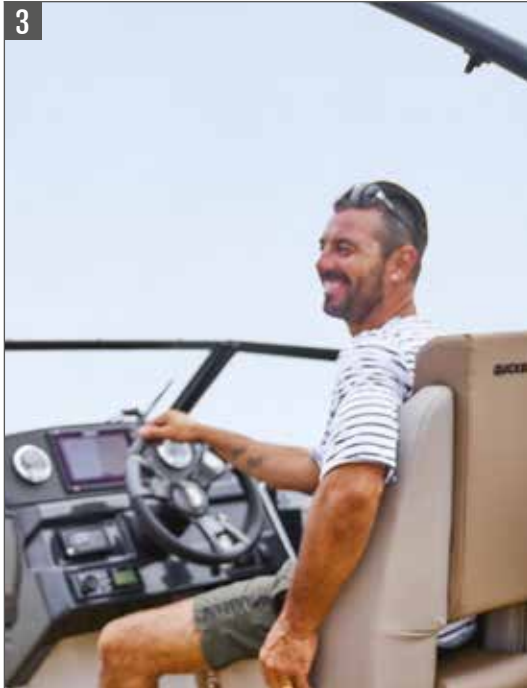
Ergonomic helm with SmartCraft instrumentation with mounting space for optional GPS/Chart plotter
