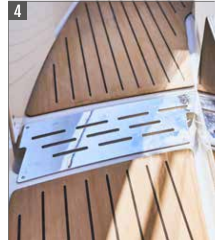
Drain system to avoid water accumulation
